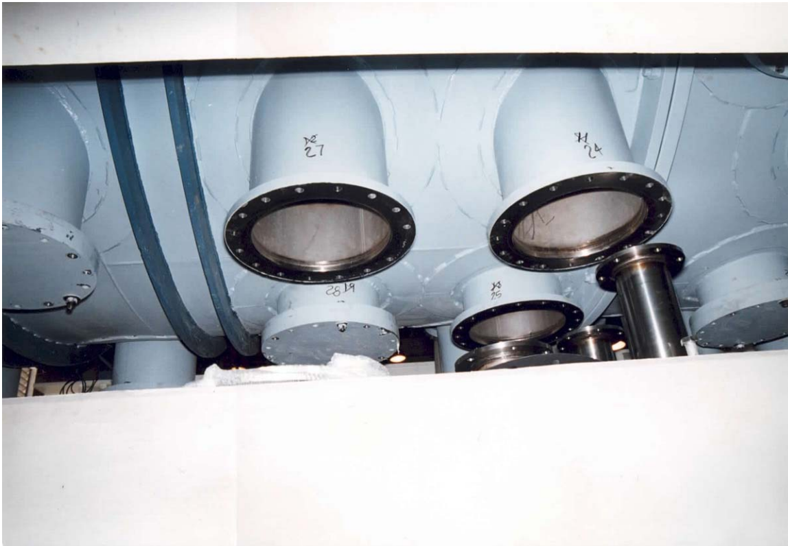
Underside view of the vacuum chamber. Thirty (30) chamber flanges protrude downward toward the mass. Adjustable "stand-offs" on the mass attach to the chamber at the flanges using a flexible vacuum seal.
