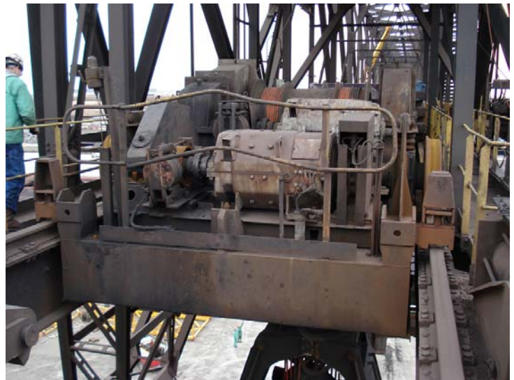
The clam bucket (at left) that scoops the ore pellets weighs approximately 20 tons when full. This is attached to the trolley that moves over the rail (below).
