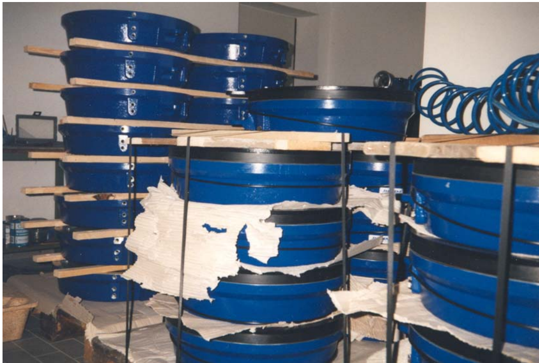
Twenty-four (24) large concrete reaction masses are isolated on a total of 248 pneumatic isolators.
