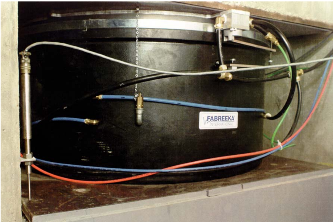
An LVDT (displacement transducer) is installed at each corner of the inertia mass. The LVDT's monitor the exact position of the mass/standoffs and platform to within 0.001 inch.
